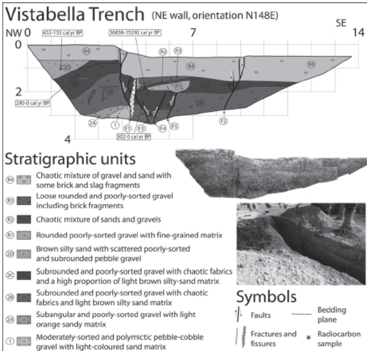
Fig. 4: Log and photomosaic of backhoe trench dug across the graben depression in Vistabella Park and image of the trenching site showing the scarp associated with the master fault.
