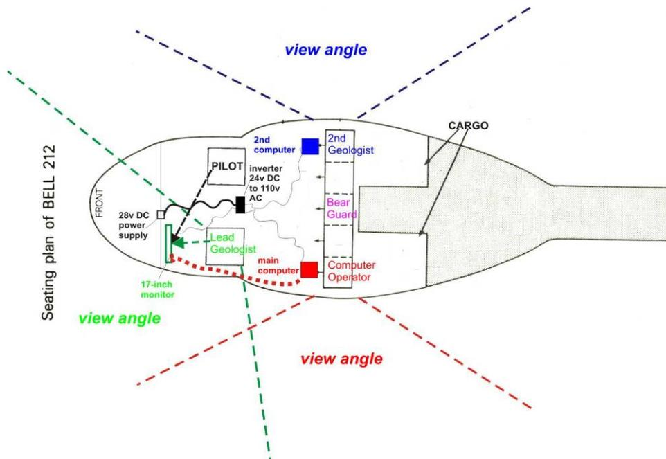
Fig. 5. Interior arrangement of the aerial mapping team in a Bell 212 helicopter. Green, blue, and red indicate the stations and view angles of the Lead Geologist, 2<sup>nd</sup> Geologist, and Computer Operator.
